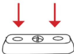
When installing the Safedock use the dock holes as a guide when drilling.
