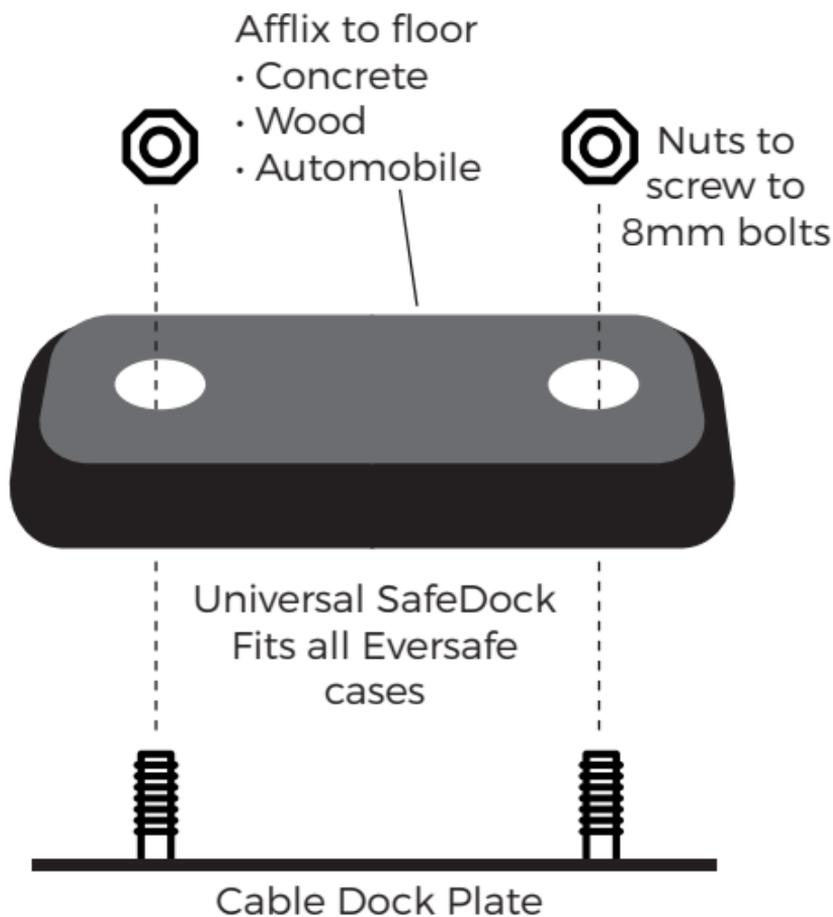
Docking plate is attached to SafeDock using 2 8mm bolts. ( assembled at factory - for information only)
