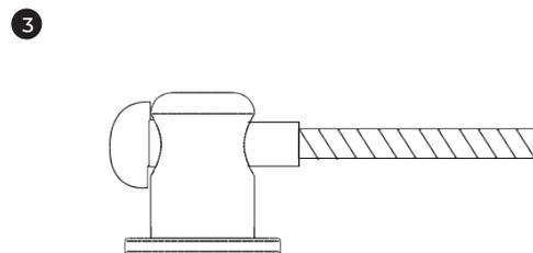
The wider cable swage will stop the cable from coming through all the way
