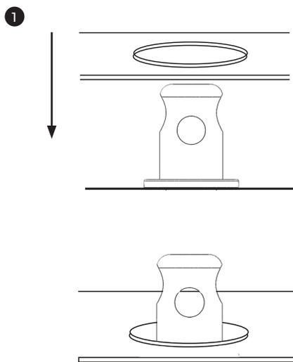
Pull the zipper cover over the zip inserting the pillars into the eyelets
