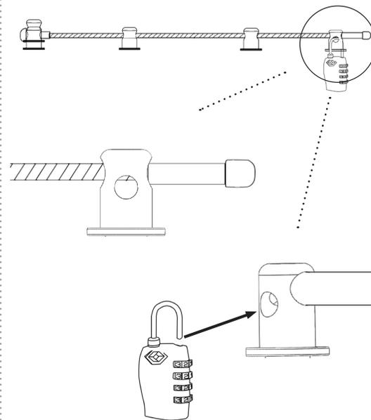
Once the cable has come through all four pillars lock the cover in place at the pillar containing two holes with the four digit combination lock
