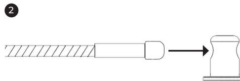
Insert the cable through all four pillars. Feed the cable through the pillar with two holes last.
